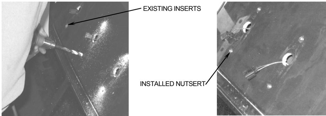
3. Feed harnesses through bracket tubes. Fasten the brackets to the installed nutserts using the supplied 1/4 x 1 hex head bolts, lock-washers and flat-washers, according to their marked orientations as follows:
