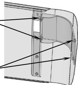
14. Install clearance lights using supplied 8-32 x 1" pan head bolts and hex nuts onto sunvisor, covering rectangular holes and brackets.
