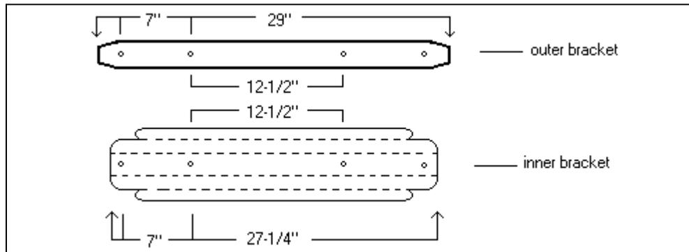
3. Hold inner (inside cab) support bracket in place over center post of windshield and drill two center holes to line up with outer support bracket.
