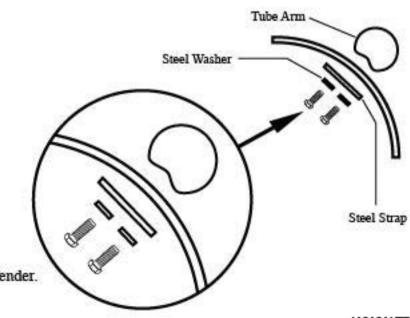
Place Tube arm to fenders as shown. Attach bolts with strap on the underside of fender.
